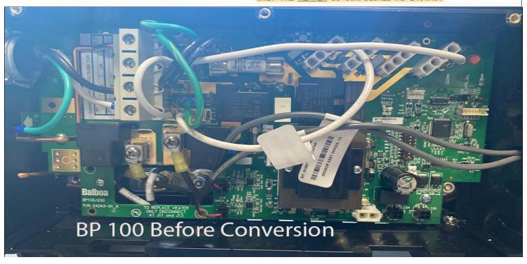
1. Swap the F3 fuse with the one included on the back of your power system. Save the removed fuse in the pouch in case you want to convert back later. only do this step if a fuse is included, if a fuse is not included, you can skip this step as your pack is already good to go.
