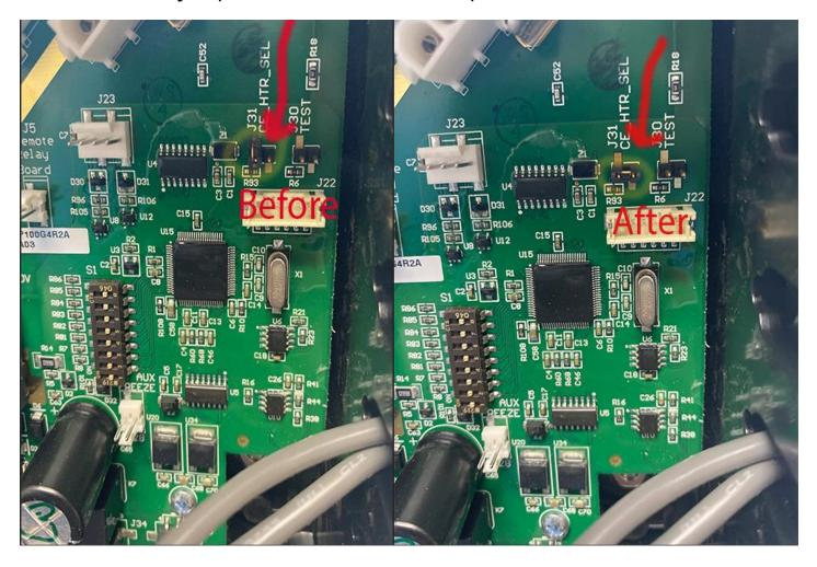
3. Remove one of the J24 jumpers. Position the other one over the two middle pins.
