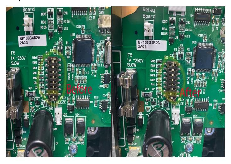
5. Remove jumper wire from area 1 (J4) to area 3 (J20) to clear a spot in area 1. Move jumper wire on J46 from area 3 (J10) to area 1(J4)
